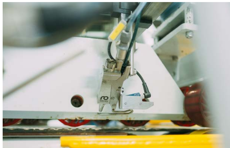
Application of SpeedUp creasing fluid at packaging manufacturer Solpap.
