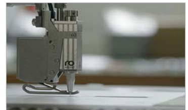
Sempre for bead application for bottom and side gluing
